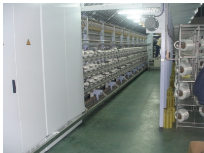
The yarn is respooled several times in order to ensure consistent tension
