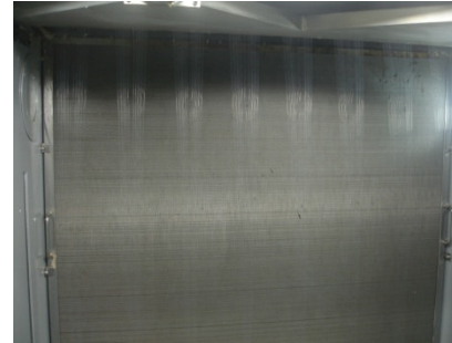
The fibers are flowing through multiple floors to control temperature and thickness
