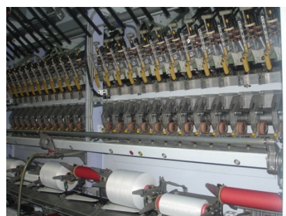
The last respooling involves the yarn being spooled from side to side
