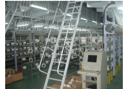
The temporary spools are stored before being respooled
