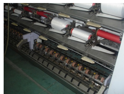
The spool is then built to a consistent diameter
